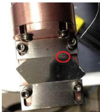
Figure 15: The sample holder with a sample held by two horizontal metal clamping strips. The thermocouple is clamped between the front sample surface and the upper clamping strip in order to measure the temperature of the sample surface accurately.
