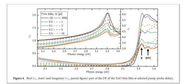
ellipsometry. The peak around 3.35 eV comprises the excitonic transitions (X) and the peak around 3.42 eV is associated with exciton–phonon complexes (EPC) [36]. There exist also further complexes at slightly higher energy.
