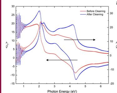
Ultrasonic cleaning, first with water then with isopropyl alcohol.
