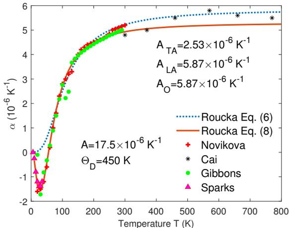
FIG. 3. Linear thermal expansion coefficient  $\alpha$  versus temperature taken from the literature<sup>35–38</sup> (symbols) along with a fit to the data using Eq. (25) (dotted) and Eq. (27) (solid).
