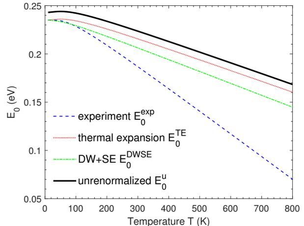
FIG. 4. Direct gap  $E_0$  of InSb versus temperature. Dashed: experimental gap  $E_0^{\text{exp}}$  from Eq. (28); dotted: thermal expansion contribution; dot-dashed: Debye-Waller and self-energy contributions from Eq. (29); solid: unrenormalized band gap from Eq. (24) for calculation of effective masses.
