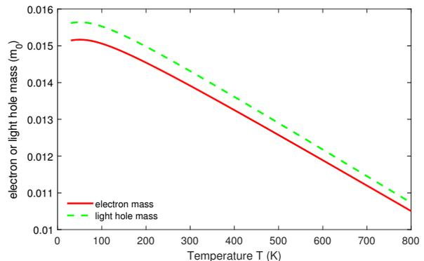
FIG. 5. Effective masses of the electron (solid) and light hole (dashed) bands of InSb as a function of temperature, calculated taking into account only the thermal expansion contribution to the band gap shift, not the Debye-Waller and self-energy terms.
