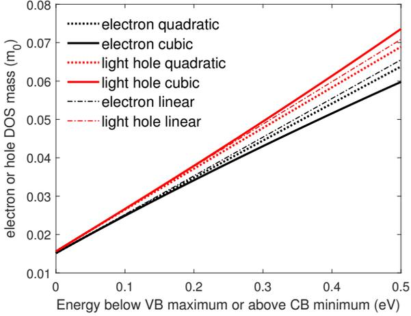
FIG. 6. Effective density of states electron mass  $m_{e,\text{DOS}}^*$  (black) and light hole mass  $m_{lh,\text{DOS}}^*$  (red) of InSb at 0 K as a function of excess energy above the conduction band minimum or below the valence band maximum, calculated from Eq. (39) (solid). The dotted lines show the results with  $\beta_n=0$ . The dash-dotted lines show the linear expansion (40).
