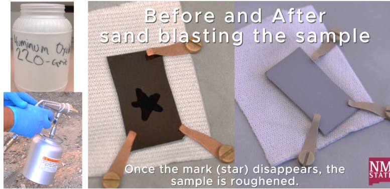
Fig. 9: Image shows the aluminum oxide (top left), sandblaster (bottom left), and the change in reflection before and after sandblasting the sample. The photographs were captured by the research group.
